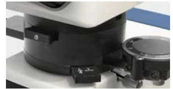
Bertrand lens, \lambda Slip, 360° rotatable analyser (removable)
