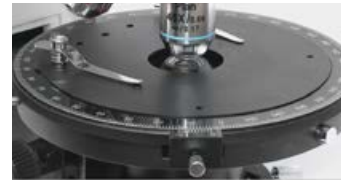
Center-adjustable and turnable polarisation stage
