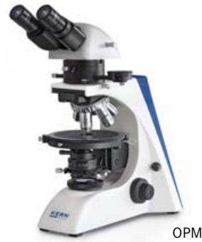
Bertrand lens, \lambda Slip, 360° rotatable analyser (removable)
